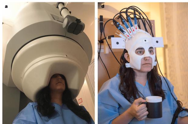
Current MEG scanner based on SQUID sensors
